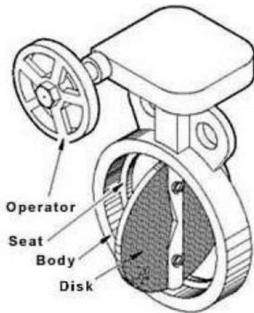
The discs in standard butterfly valves are quite narrow and occupies little space in the pipeline. The shaft is centered on the axis of the pipeline and is in line with the seal.
